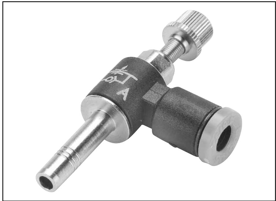
Plug-in flow control regulators can be directly mounted into existing fittings and allow very compact installations. They are particularly suited for mounting in manifolds using cartridges. Their design and function give equal performance to that of flow control regulators with threaded connections.
