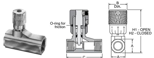
**338 Bi-directional Flow Control Valves - BSPP**
