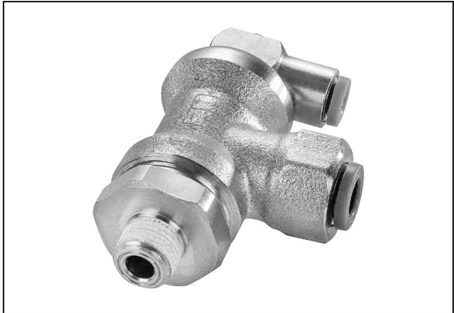
Blocking valves prevents damage to work and equipment in the event of a loss of pressure. Blocking valves which are mounted in pairs on a cylinder lock the piston by simultaneously cutting off the supply and exhaust. Functional locks are more precise and rapid when blocking valves are located on the cylinder: the volume of air in the pipework no longer needs to be taken into consideration.
