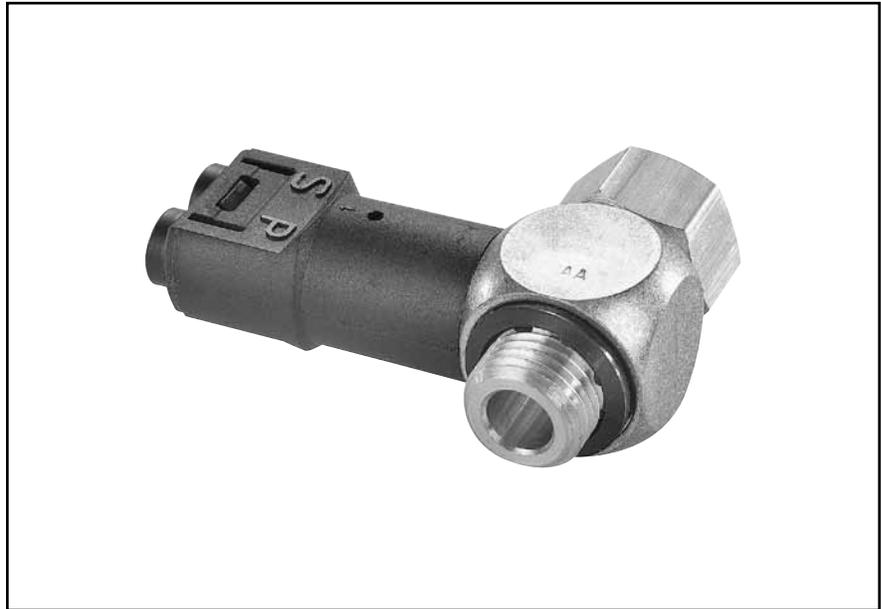
The sensor fitting detects the absence of pressure and translates it to a high pressure pneumatic output. When used to monitor the decaying or exhausting side of a pneumatic cylinder's piston, it emits a positive output. When the cylinder comes to the end of its stroke, wherever that may be, the signal emitted from the sensor can then be used to pilot the next step.
