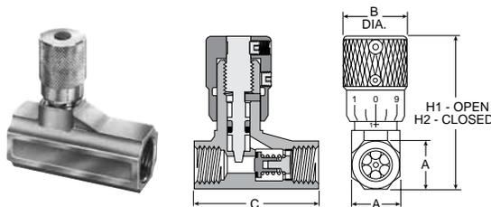
**337 Micrometer Flow Control Valves - BSPP**
