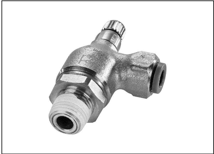
Metal flow control regulators are suited for use in severe conditions (temperatures, sparks, abrasion, etc). The screw and locking nut have been designed for easy manipulation, by hand. Adjustment can be made with a screwdriver and locking by use of a wrench.
