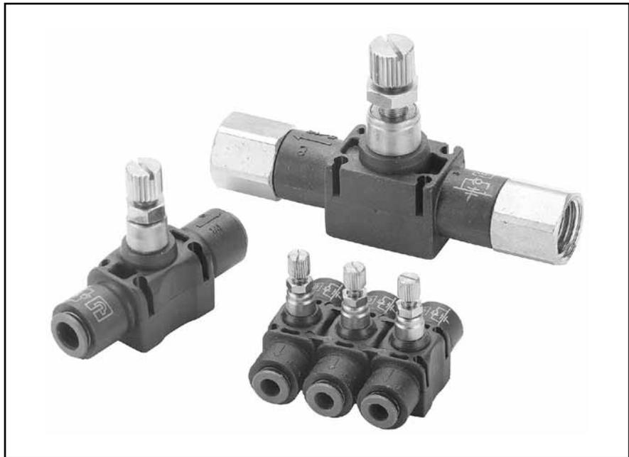
In-line flow controls are unidirectional flow control valves. Intake air flows freely through the flow control; exhaust air is metered out through a specially designed adjustment screw. An arrow on the body of the valve indicates the direction of controlled flow. They can be easily added to existing circuitry. Simply splice it into the cylinder port line.
