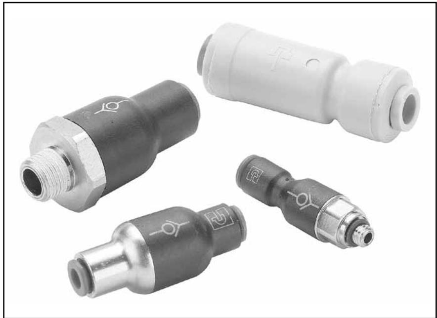
These in-line check valves allows air to pass in one direction while blocking flow in the other direction. Their extreme compactness and light weight make them suitable as a safety item in compressed air circuits. The body of the fitting contains an arrow to indicate the direction of flow.
