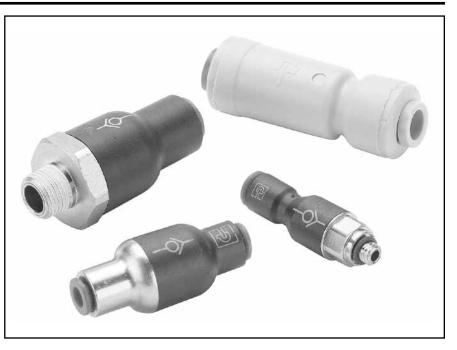
These in-line check valves allows air to pass in one direction while blocking flow in the other direction. Their extreme compactness and light weight make them suitable as a safety item in compressed air circuits. The body of the fitting contains an arrow to indicate the direction of flow.
