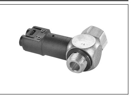
The sensor fitting detects the absence of pressure and translates it to a high pressure pneumatic output. When used to monitor the decaying or exhausting side of a pneumatic cylinder's piston, it emits a positive output. When the cylinder comes to the end of its stroke, wherever that may be, the signal emitted from the sensor can then be used to pilot the next step.
