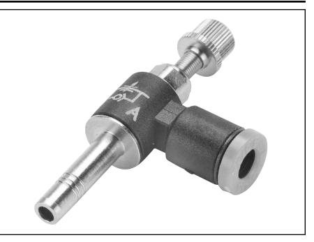
Plug-in flow control regulators can be directly mounted into existing fittings and allow very compact installations. They are particularly suited for mounting in manifolds using cartridges. Their design and function give equal performance to that of flow control regulators with threaded connections.
