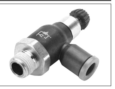
Compact flow control regulators ensure excellent performance of flow and are perfectly suited for reduced spaces due to their small size. The sensitivity of the adjustment screw provides very precise air flow control and regulation. A locking nut guarantees stability of adjustment against vibration tampering of the flow setting.
