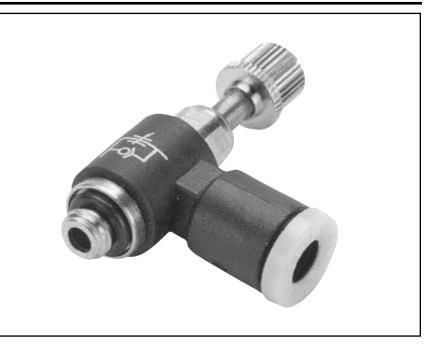
The miniature flow control regulator is especially adapted for all very small sized pneumatic applications (micro-pneumatic in particular). They are specifically designed for use with small bore cylinders (pancake / flat cylinders). Miniature flow control regulators are available in meter out, meter in and bi-directional versions.
