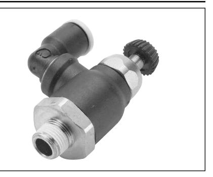
Flow control regulators with "swivel outlet" are especially designed to allow a vertical or angled tube exit where access is restricted. The swivel outlet comes with instant push-in connection to ease installation. Flow control regulators with swivel outlet are available in meter out and meter in versions.
