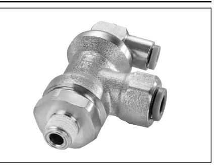
Blocking valves prevents damage to work and equipment in the event of a loss of pressure. Blocking valves which are mounted in pairs on a cylinder lock the piston by simultaneously cutting off the supply and exhaust. Functional locks are more precise and rapid when blocking valves are located on the cylinder: the volume of air in the pipework no longer needs to be taken into consideration.
