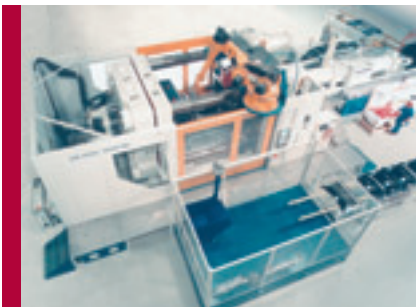
Plastics injection molding machine
