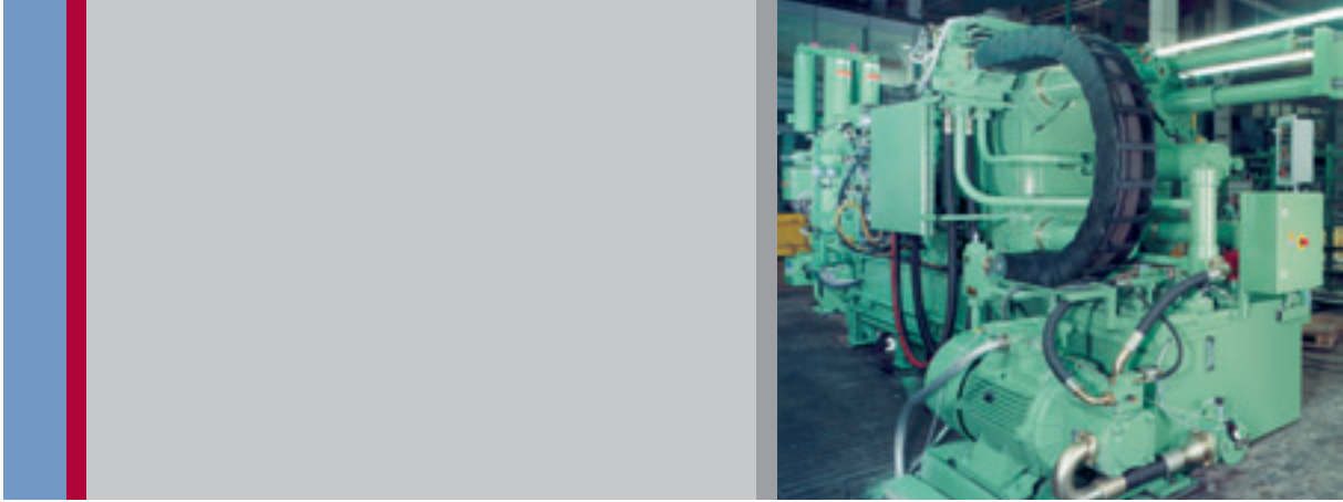
Die casting machine, pump with variable flow by speed control
