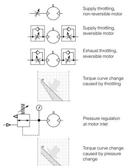
The most common way to reduce the speed of a motor is to install a flow control valve in the air inlet. When the motor is used in applications where it must reverse and it is necessary to restrict the speed in both directions, flow control valves with by-pass should be used in both directions.
