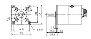
Note: A foot plate can be fitted turned by steps of 90° from the original position
