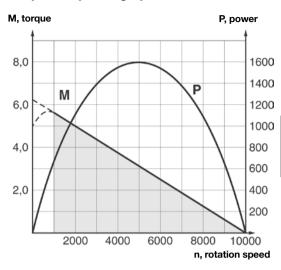
There is a graph for each motor, where torque and power can be read off as functions of speed. When the motor is stationary without air and when it rotates without load on the output spindle (free speed), it does not develop any power. Maximum power is normally developed when the motor is braked to half the free speed.
