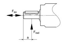
Fig. 1: Loading on output shaft.
