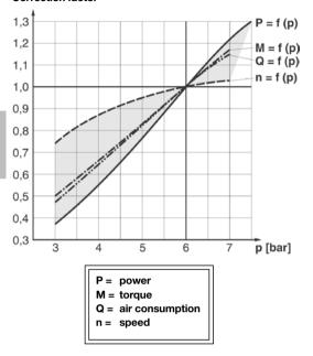
All catalogue data and curves are specified at a supply pressure of 6 bar to the motor. This diagram shows the effect of pressure on speed, specified torque, power and air consumption.
