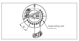
2. Then, rotate the fine adjust screws on the reference point stopper and the angle setting stopper until the correct angle is obtained. After completing the angle setting, the locknut must be tightened.
