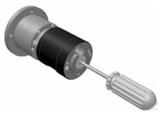
**Step 4.**Remove the old vane and replace it with a new one.
