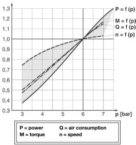
All catalogue data and curves are specified at a supply pressure of 6 bar (in the inlet port). This diagram shows the effect of pressure on speed, torque, power and air consumption.
