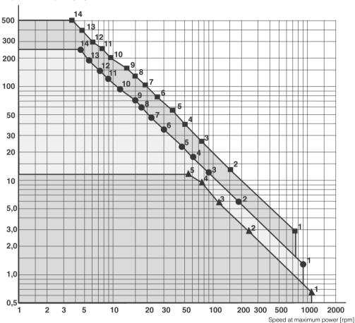
The motor to be used should be selected by starting with the torque needed at a specific shaft speed. In other words, to choose the right motor, you have to know the required speed and torque. Since maximum power is reached at half the motor's free speed, the motor should be chosen so that the oprating point is as close as possible to the maximum power of the motor.
