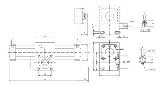
The location of the shaft key is indicated when the pistons are on the left. First rotation as indicated (clockwise).
