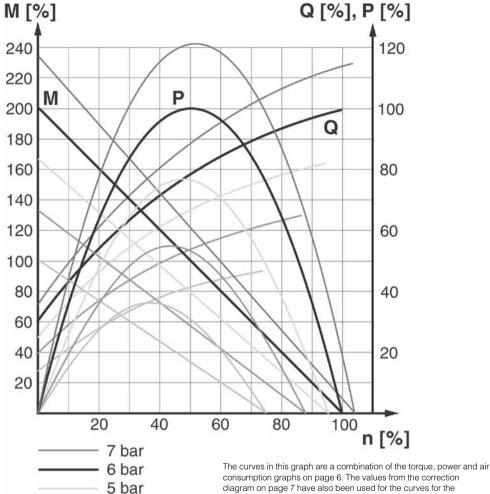
P = power Q = air consumption M = torque n = speed
