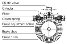
turned out by pushing force of coiled spring and release conducted by air pressure as usual. Brake shoe is opened from drum as piston for release works after air pressure is applied to supply port of air motor and simultaneously to brake cylinder.
