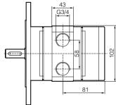
Dimensions (mm) Motor P1V-A360A0600 Flange IEC 90 A B5
