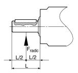
Fig. 3: Force applied at centre of shaft
