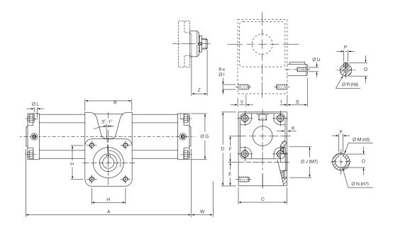
The location of the shaft key is indicated when the pistons are on the left. First rotation as indicated (clockwise).
