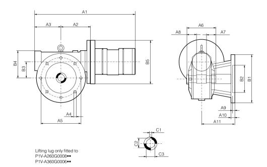
As standard, the motor has a hollow shaft with key slot.
