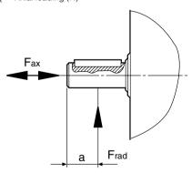
Fig 1: Load on output shaft for basic motor with shaft with key slot.
