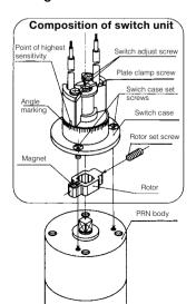
Mount the switch unit on the body using the set of screws. For clamping torque, refer to the table below :
