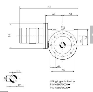
As standard, the motor has a hollow shaft with key slot.
