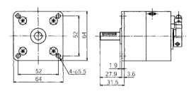
**Note :** A foot plate can be fitted turned by steps of  $60^{\circ}$  from the original position
