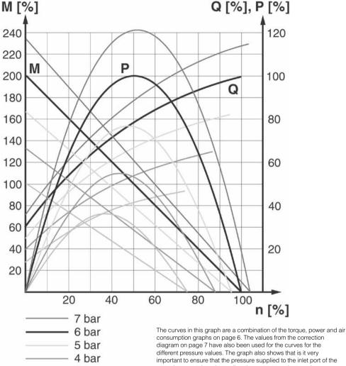
P = power Q = air consumption M = torque n = speed
